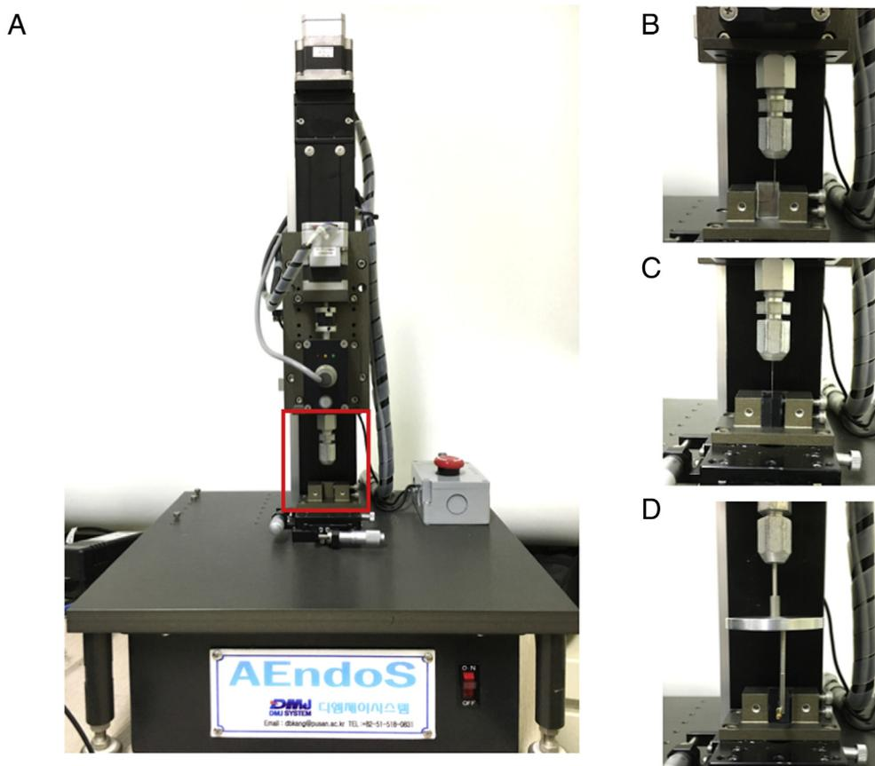
**Figure 1.** The devices used in this study. (A) The custom device used for the test (AEndoS), (B) a jig and simulated canal used for the cyclic fatigue test, (C) a jig and polycarbonate resin blocks used for the torsional resistance test, and (D) a jig and loading part used for the bending stiffness test.
