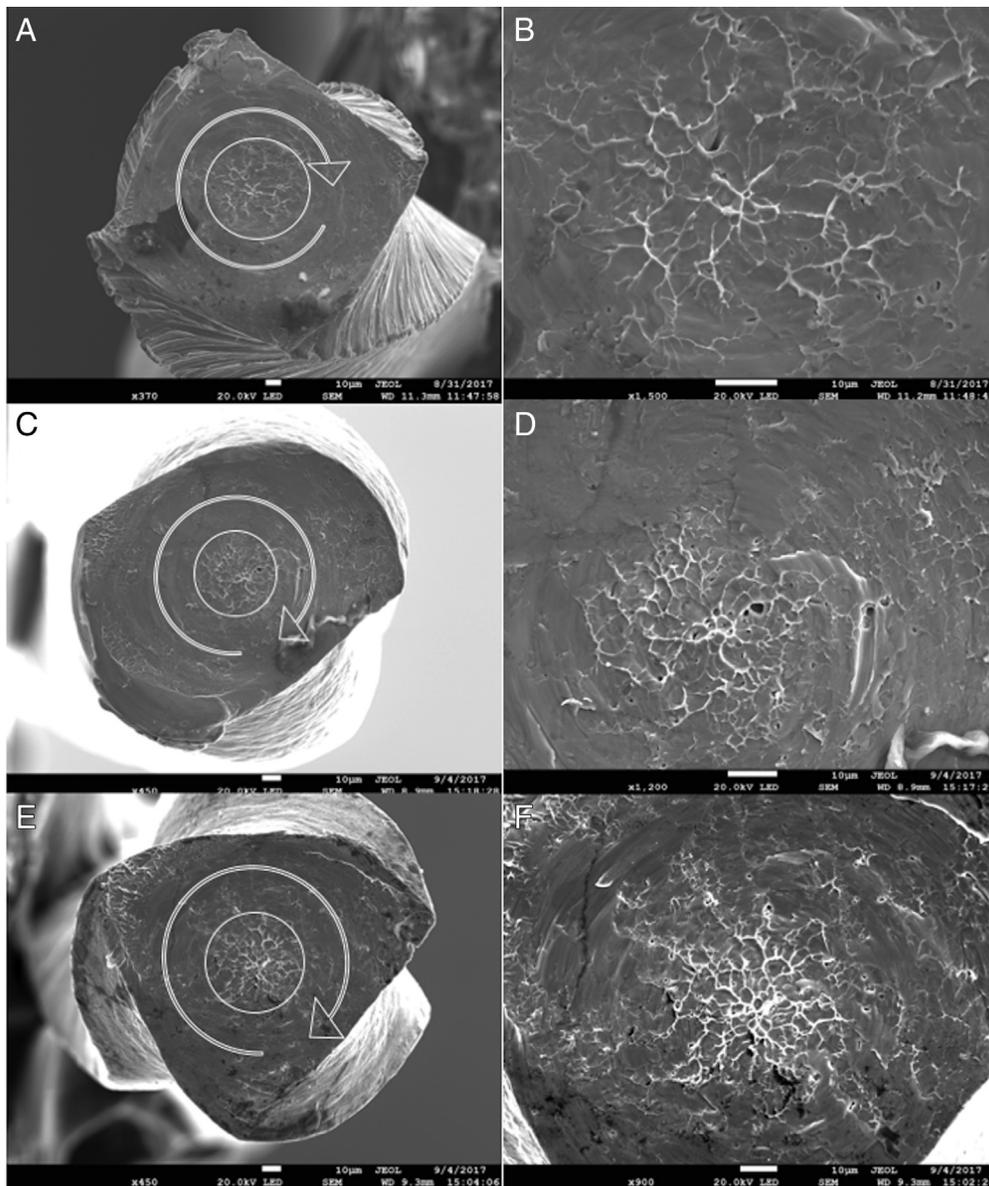
**Figure 3.** Representative scanning electron microscopic images (cross-sectional aspects) of the fractured surfaces of the separated instruments after the torsional resistance tests. The *circle arrows* indicate the circular abrasion marks, and the *full circles* indicate skewed dimples near the center of rotation ([A] PG, [C] OG, and [E] EG). The magnified views in the right column show numerous ductile dimples (B, D, and F are the magnified views from A, C, and E, respectively).
