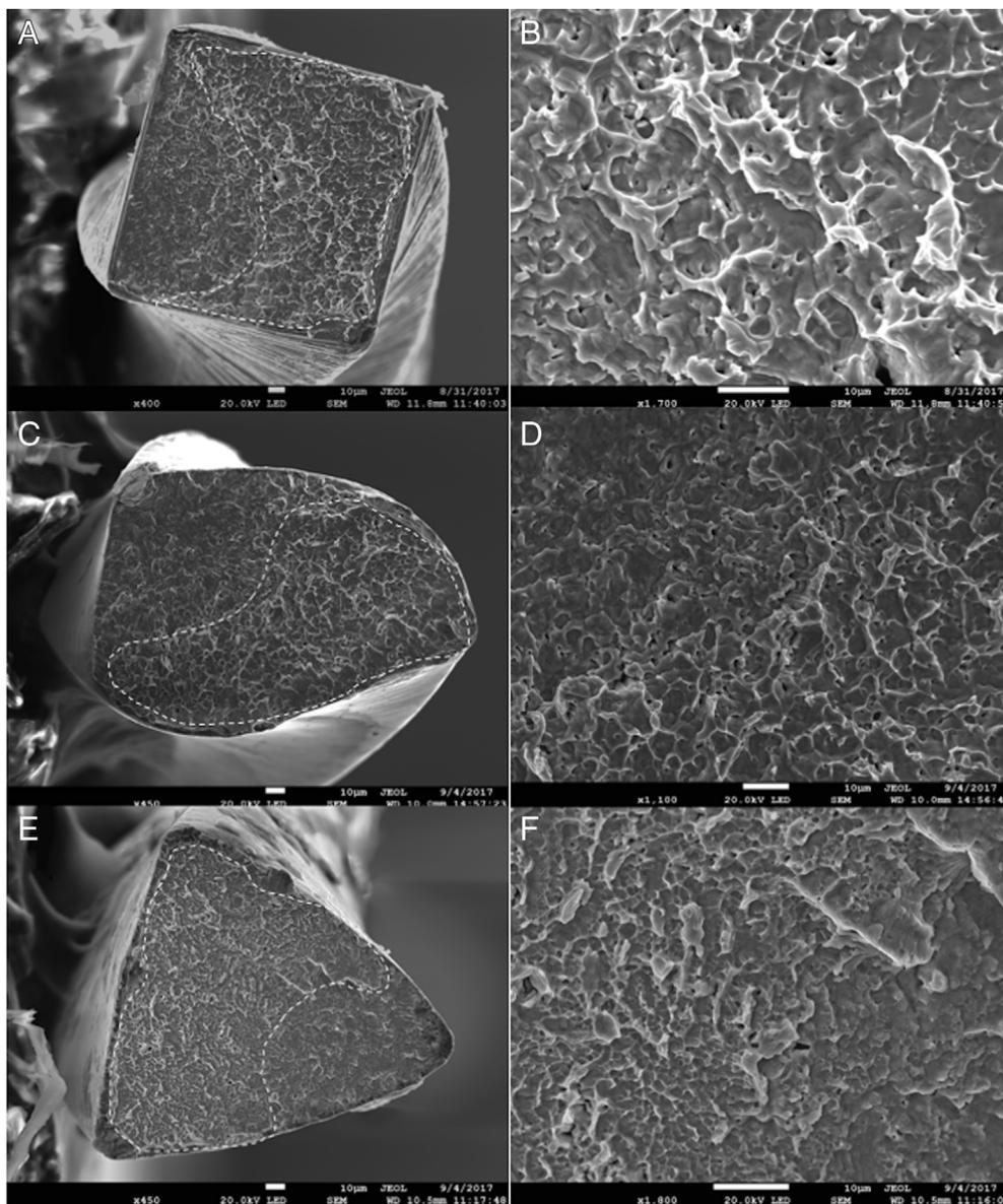
**Figure 2.** Representative scanning electron microscopic images (cross-sectional aspects) of the fractured surfaces of the separated instruments after the cyclic fatigue tests. The *dimpled area outlined with the dotted line* indicates an overload fast fracture zone ([A] PG, [C] OG, and [E] EG). The magnified view shows an overload fast fracture zone with numerous ductile dimples (B, D, and F are the magnified views from A, C, and E, respectively).
